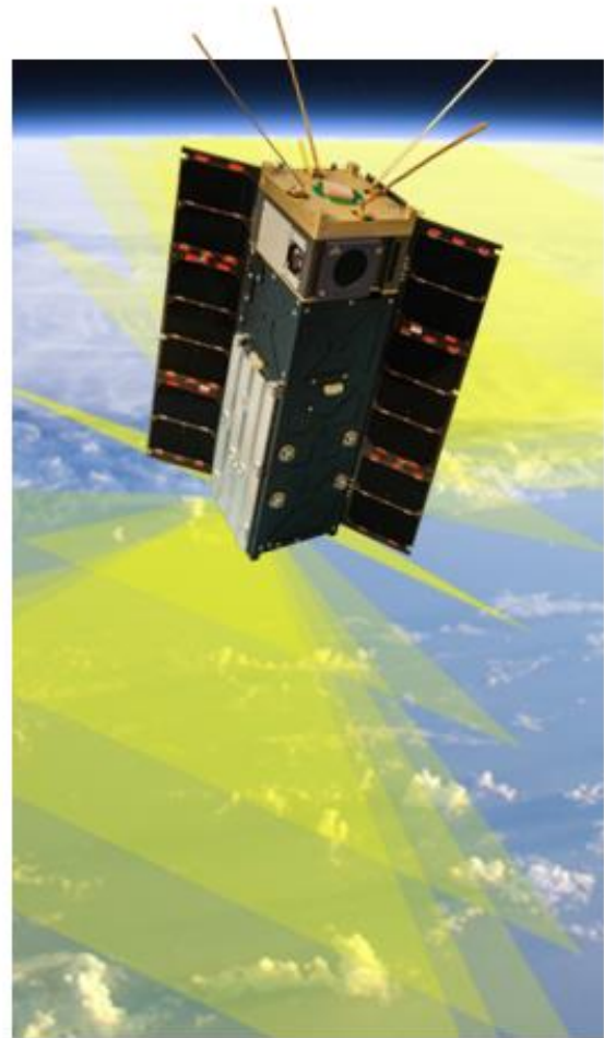
Figure 4: The HARP CubeSat spacecraft with solar panels fully deployed. Photo credit: Vanderlei Martins (UMBC/JCET)
