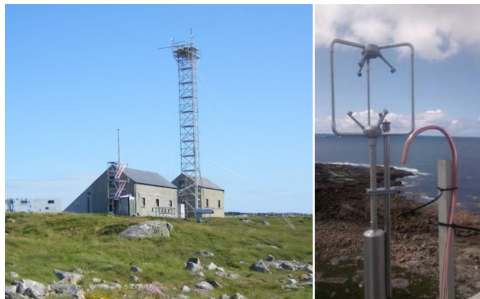
Figure 2. a) Micrometeorological Tower on the measurement observatory of Mace Head. b) Sonic anemometer and CPC inlet coupled in eddy covariance configuration.
