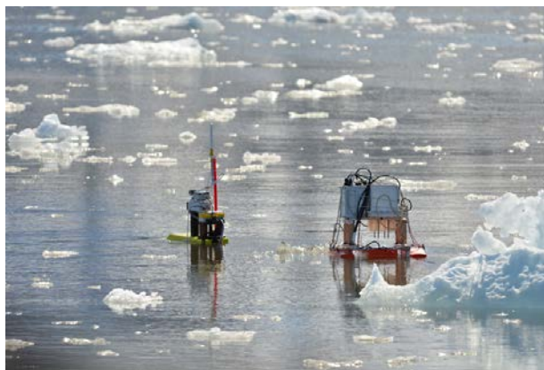
Figure 1: The automatic vehicle (left) towing the multisampler (right)
